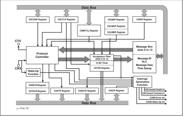
Figure 18.1 CAN Module Block Diagram
